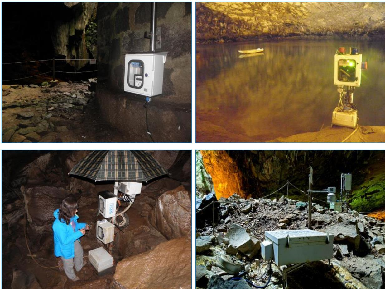
Figure 35: Monitoring, Warning and Alarm System for the Safety of Visitors to the Furna do Enxofre.
